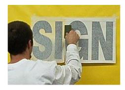
**Step 7.** Peel back the application tape slowly, making sure all of the lettering or decal is stuck to the surface.
